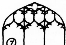
⑦ DEPRESSED OGEE SUPERMULLIONED BROOMFIELD NORTH AISLE WEST WINDOW c. 1535
